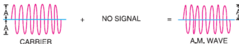
Fig: 2.4 signal with 0% Modulation
